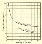
Fig. 271.—Steam consumptions of small turbines.
